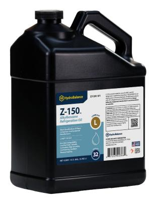
Z-150 is recommended for use with HCFC and CFC refrigerants in applications requiring a 150 SUS (ISO VG 32) alkylbenzene compressor lubricant. Do NOT use in systems with HFC refrigerants such as R134a and R410a. **Always follow the equipment manufacturer's recommendation for selection.**
